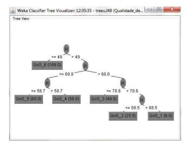
Figure 1: Tree algorithm classification used to determine the QoS, regarding the delay parameter.
