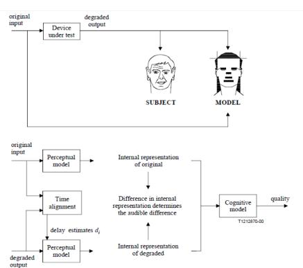
Figure 5: Algorithm used by PESQ [2].
