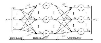
Figure 2: Perceptron network with three layers.
